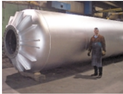
The upper end of a special Universal Silencer EN2-32 exhaust silencer for the Waltz Engineering project.
